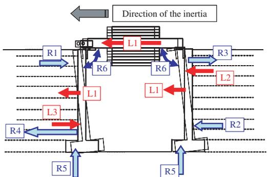
Figure 7. Load and resistance components when the inertia force of the structure is acting toward the left.
