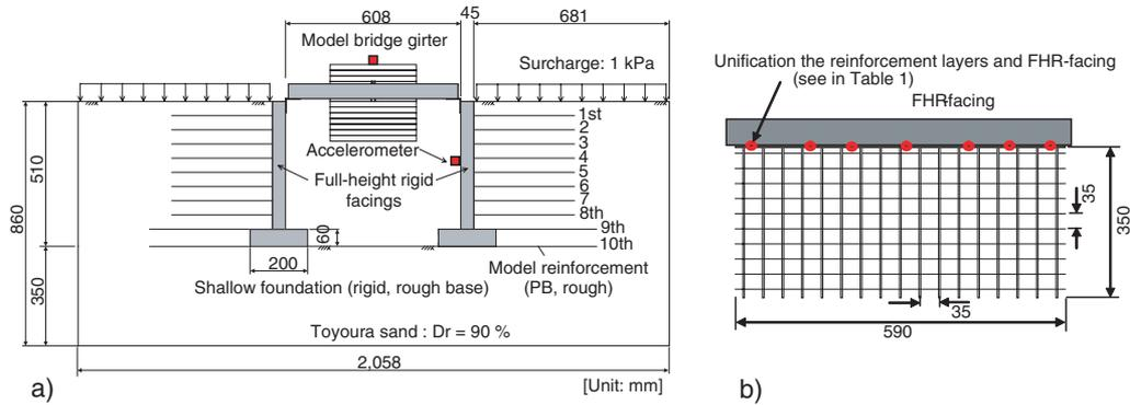
Figure 2. a) Cross-section of GRS-integral bridge model (Test 3 & 4), and b) plan of model reinforcement layer.
