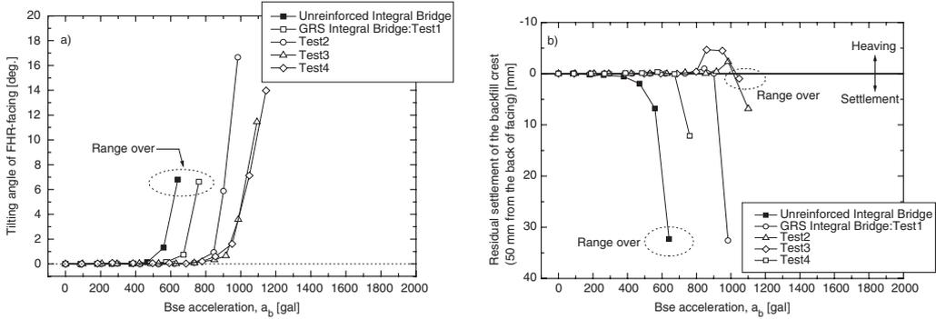
Figure 3. Relationships between base acceleration and a) residual tilting angle of the facing, and b) residual settlement of the backfill crest (50 mm from the back of facing).
