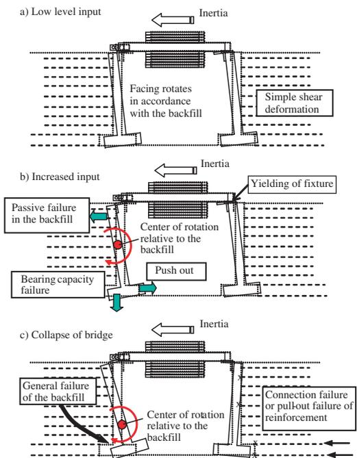
Figure 6. Failure mechanisms at different load levels.
