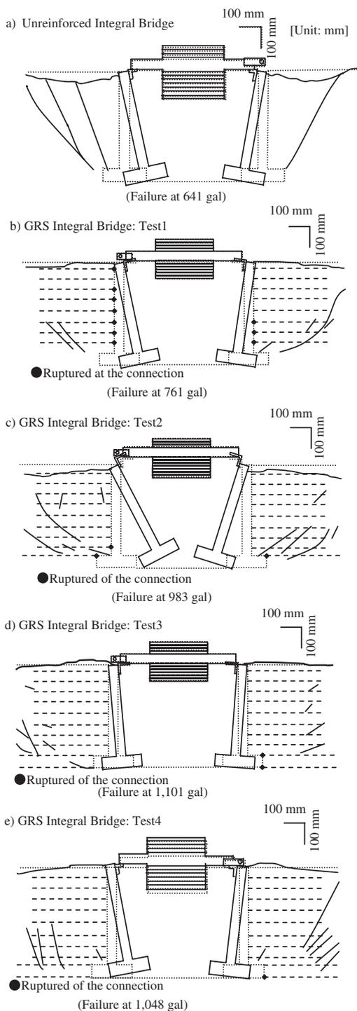
Figure 5. Failure modes of a) unreinforced integral bridge and b)-e) GRS integral bridges.
