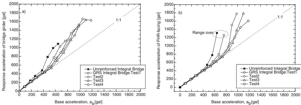
Figure 4. The relationships between base acceleration and a) response acceleration of the bridge girder, and b) response acceleration of the facing.
